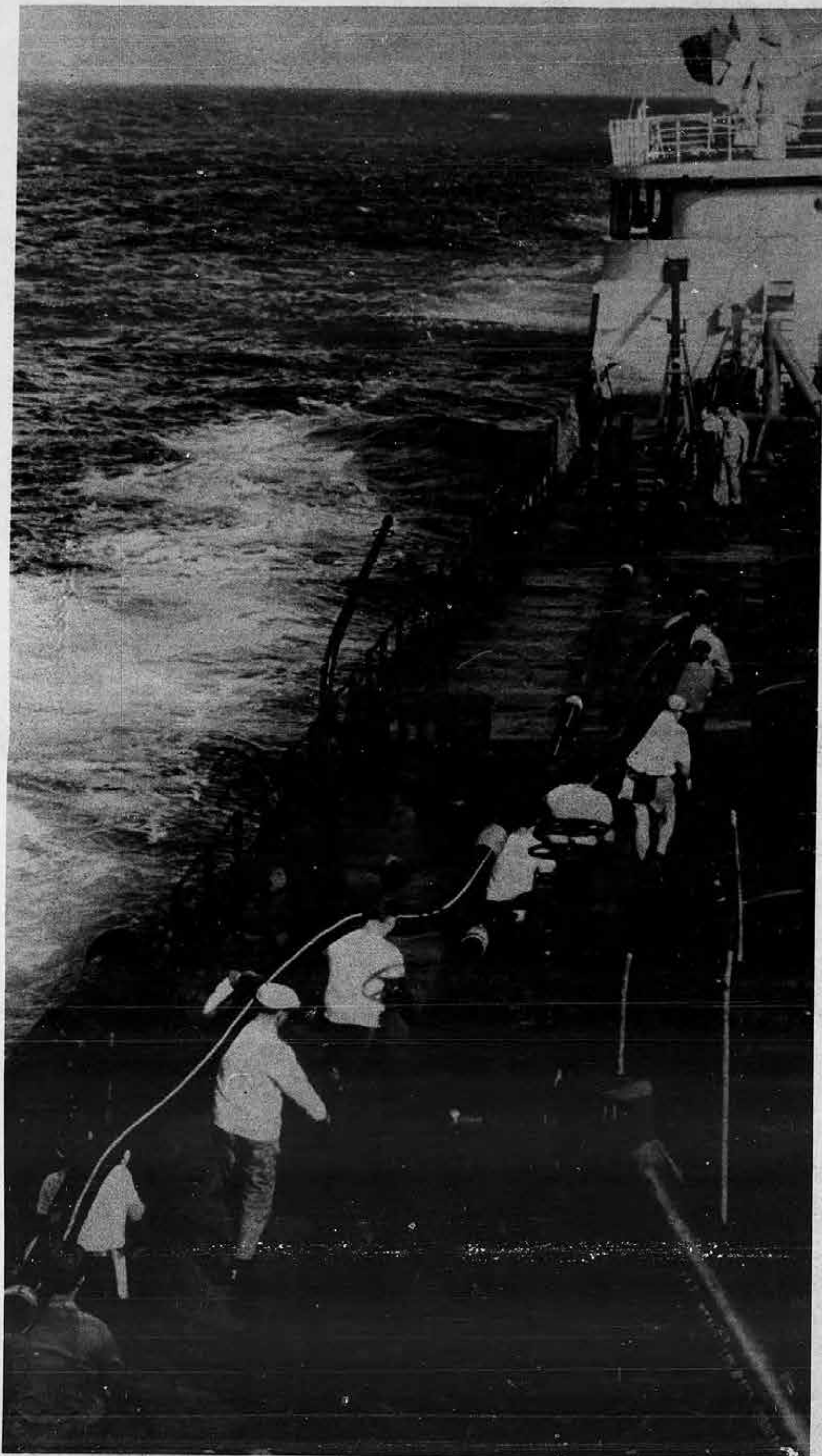
As the Erna Elizabeth makes to come alongside a navy vessel for refueling operations, crew members break out the hoses which will be used to pump oil from the SIU-contracted ship to a waiting, 'thirsty' Navy ship.
