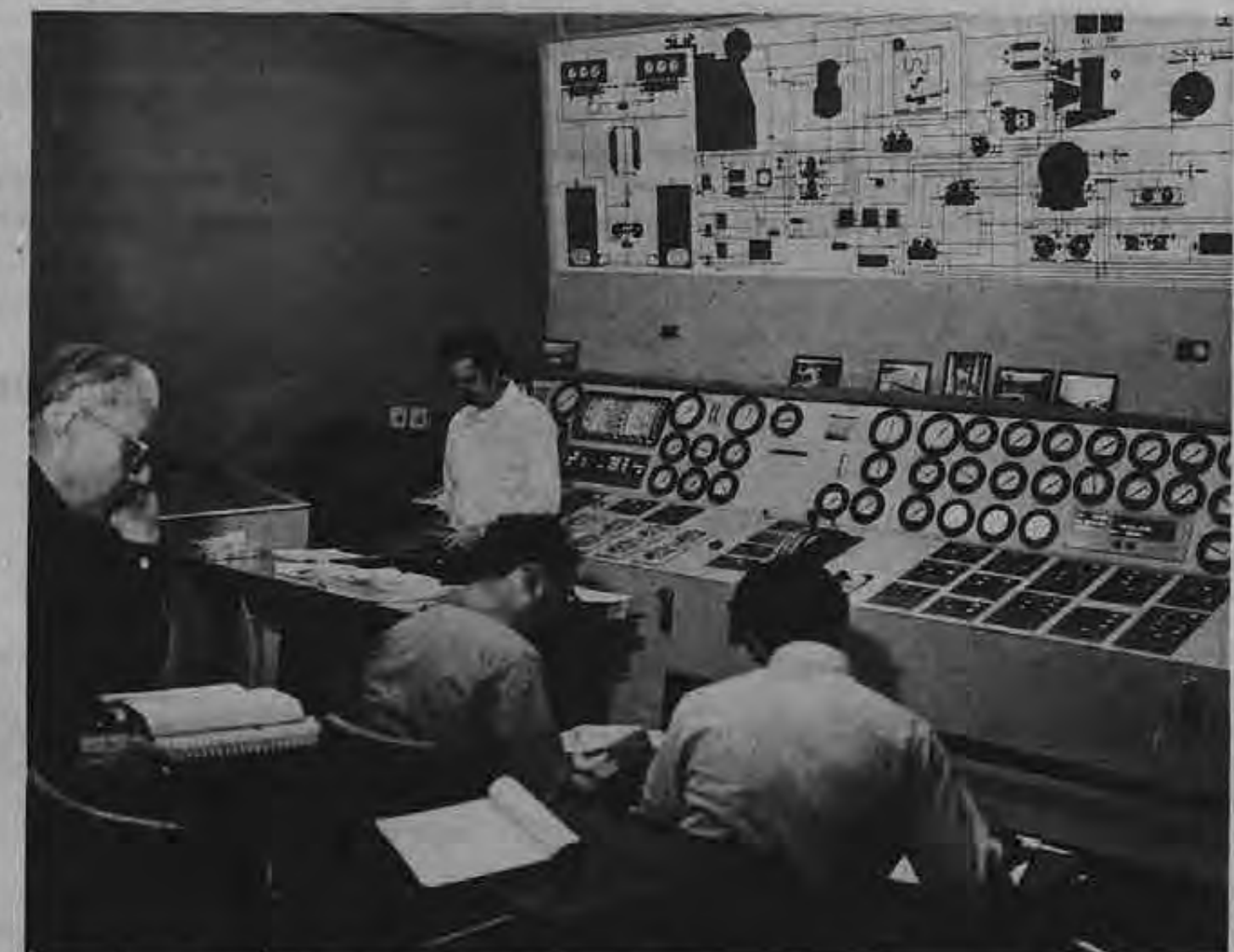
SHLSS instructor Calvin Williams reviews materials on boiler systems during a classroom session on Automation. The Automation Simulator was designed and built by the staff at SHLSS.
