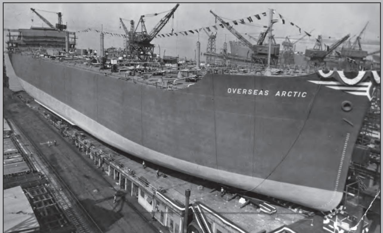
The SIU-contracted *Overseas Arctic* is pictured shortly before its launch in 1970. Built at Bethlehem Steel's Sparrows Point yard, the tanker weighed 62,000 dwt and had a capacity of 524,000 barrels. It could sail at 15.5 knots and was 731 feet long, with a breadth of 105 feet.
