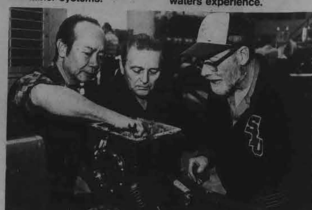
Hands-on training is an integral part of all of the upgrading programs at the Seafarers Harry Lundeberg School of Seamanship and the course in refrigeration systems is no exception. Here, three Seafarers from widely separate areas of the U.S. work together to repair a compressor. From left are Exequiel Liwag, Port of Norfolk; William Katt, Port of Chicago, and Louie Guerlin, Port of New Orleans.
