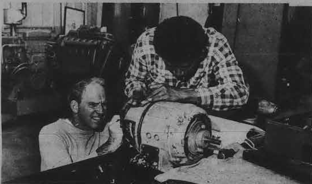
Seafarers Bob Goodrum, who ships out of the Port of Mobile, and David Terry, who sails out of Jacksonville, break down an electric motor for inspection and repair in the SHLSS machine shop.
