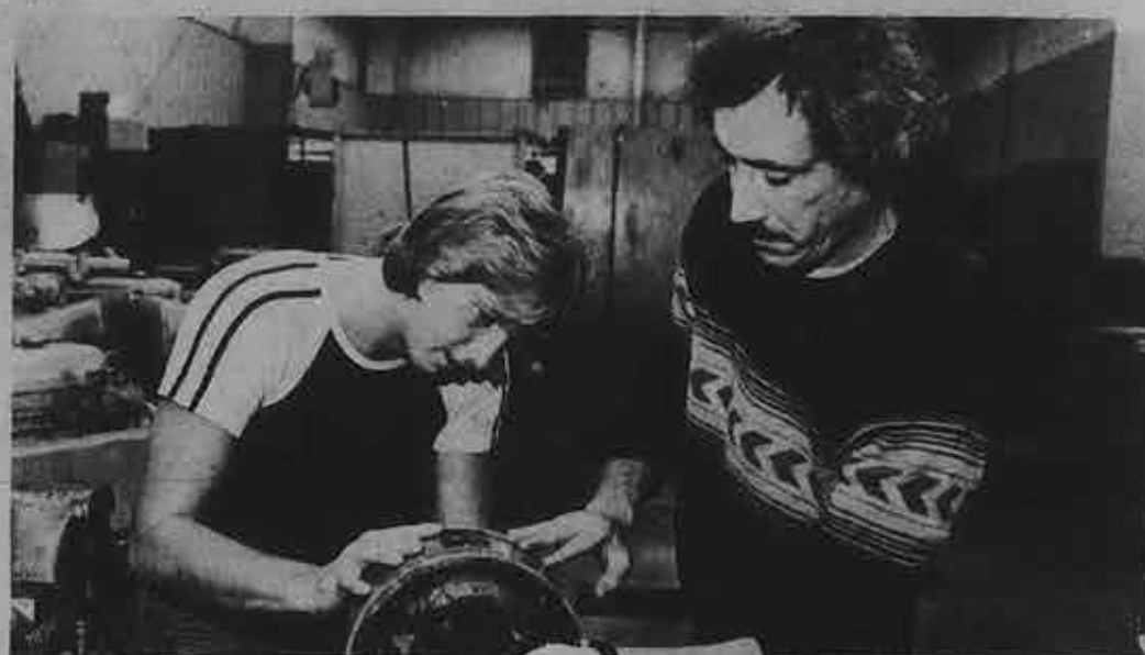
Hands-on experience is very important in all of the upgrading programs at SHLSS. Here, Seafarers Jim Pyle, from the Port of Tampa, and Dave Morgan, Baltimore, do some troubleshooting on an electric motor as part of their course in Marine Electrical Maintenance.
