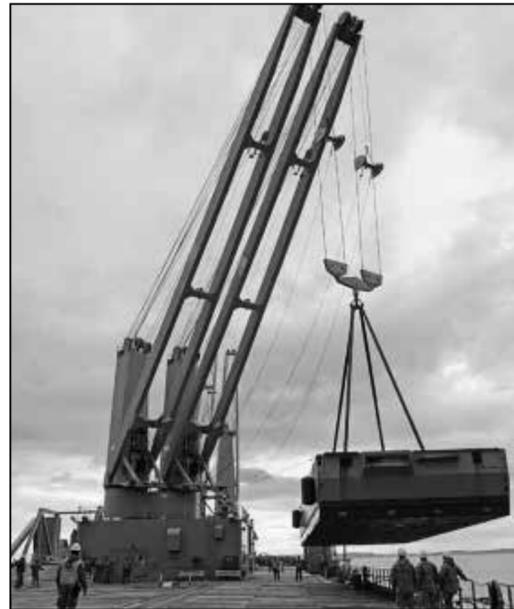
Sections of Navy lighterage are off-loaded (photo directly above) from the *USNS Bob Hope* using its deck cranes. Containerized cargo is later loaded aboard the improved lighterage system (photo at right above) prior to being moved to shore aboard a floating causeway (photo at right above). After arriving at its shoreside destination (photo below), military personnel remove the cargo from the floating causeway in preparation for transport to its final destination.
