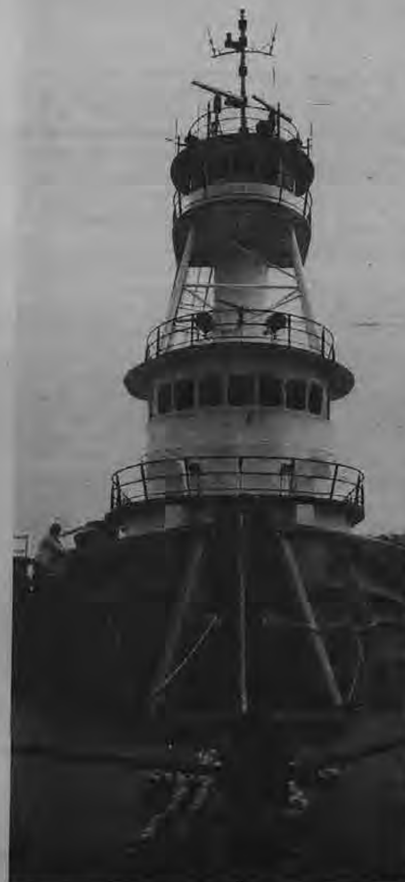
Here's a view of the tug fitting into the oil-carrying barge's slot so it can be pushed between the ports of Garyville, La., Florida, Savannah and Charleston, S.C.
