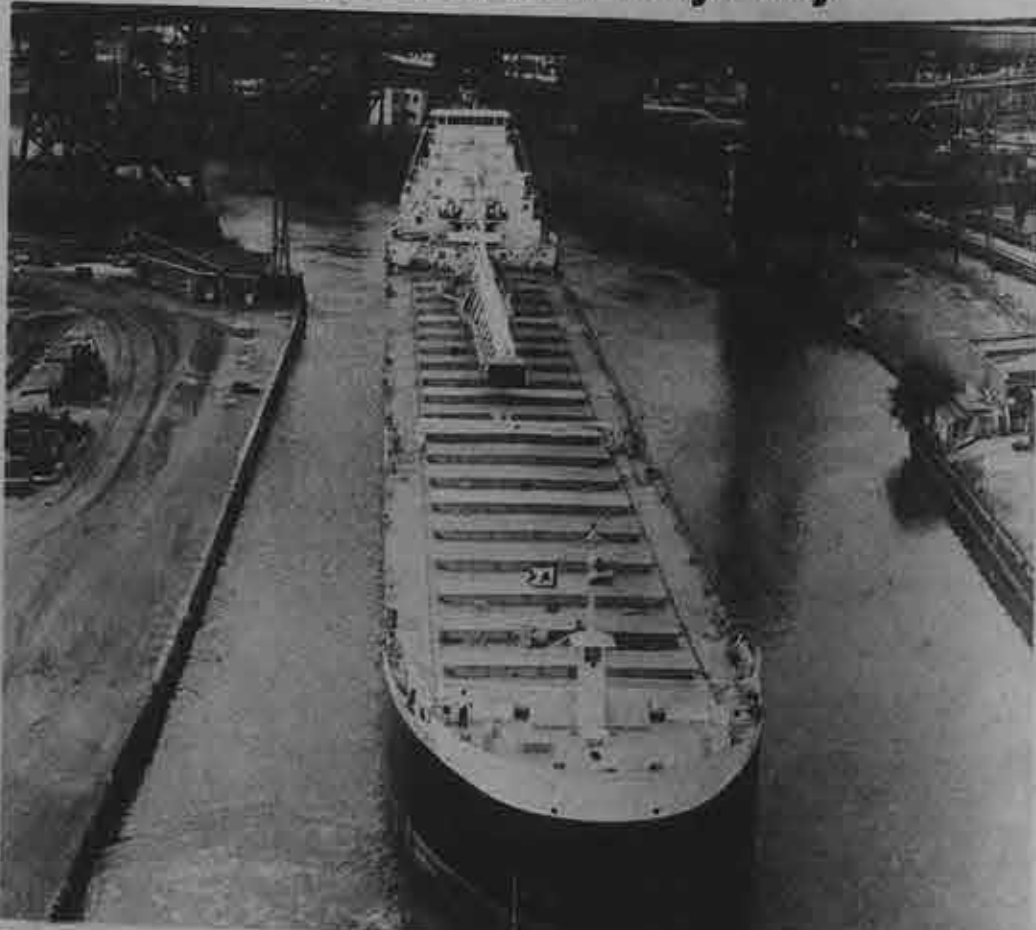
The brand new SIU-manned Great Lakes bulkier M/V American Republic makes way along Cuyahoga River in Cleveland without the support of a tug, thanks to bow and stern thrusters. The vessel was christened last month.
