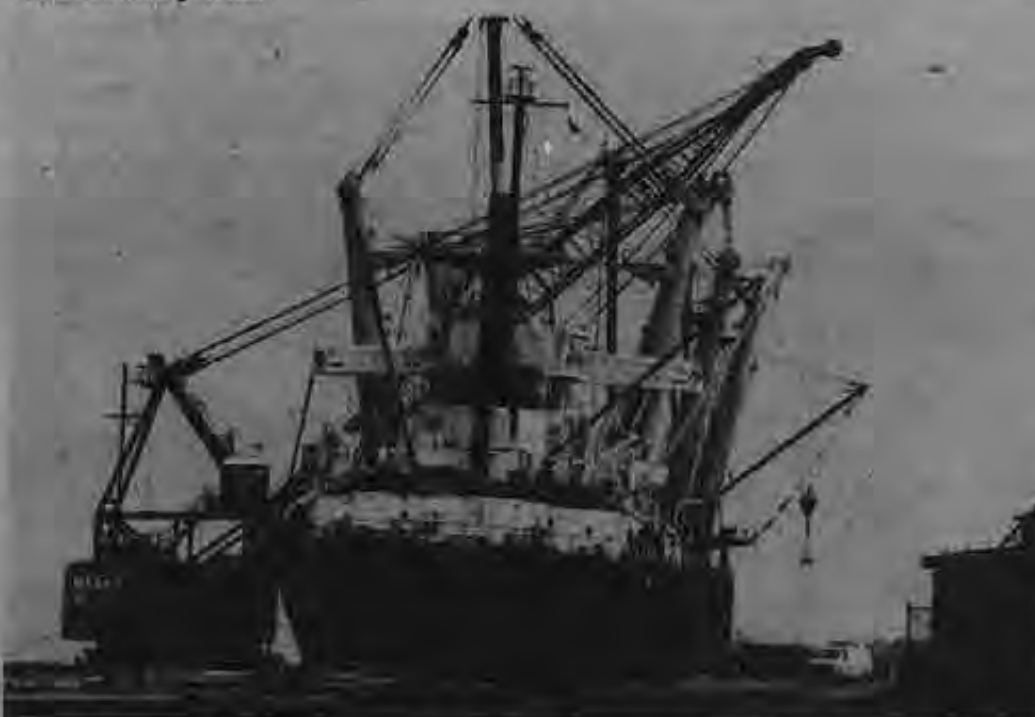
The Transcolumbia was specially outfitted with three cargo booms which are 100 feet long, weigh 45 tons and have a reach of 50 feet over the side.
