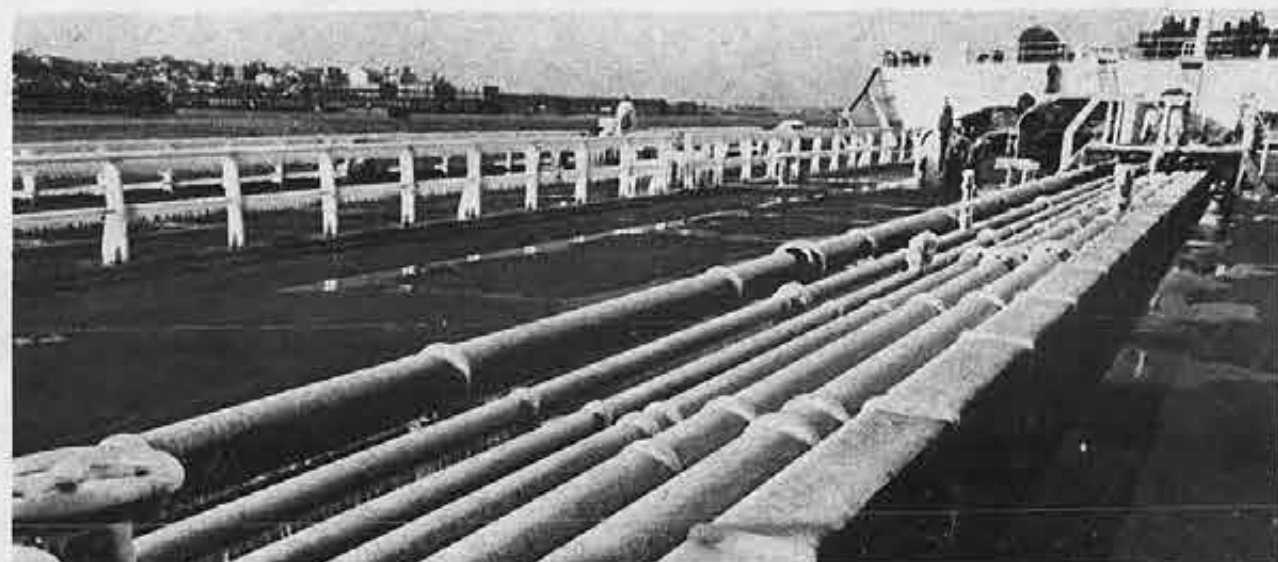
Rows of ice-covered parallel pipes topside aboard the Overseas Alaska are only part of the vessel's liquid transport system capable of carrying 524,000 barrels of oil.
