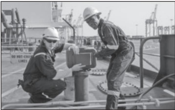
Replacing a ballast vent screen are (from left) 2M Cullen Bozza and Pumpman Lateef Sanusi.
